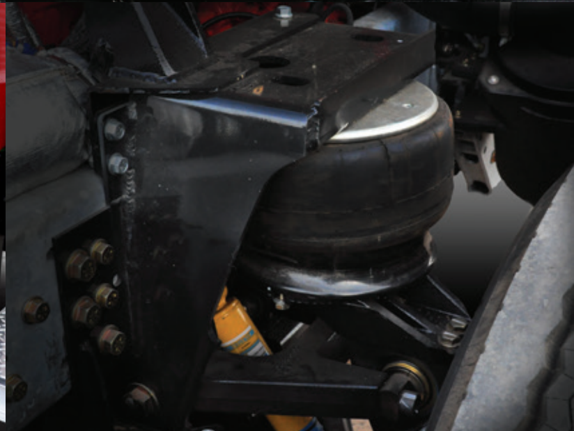
Independent Front Air Suspension
