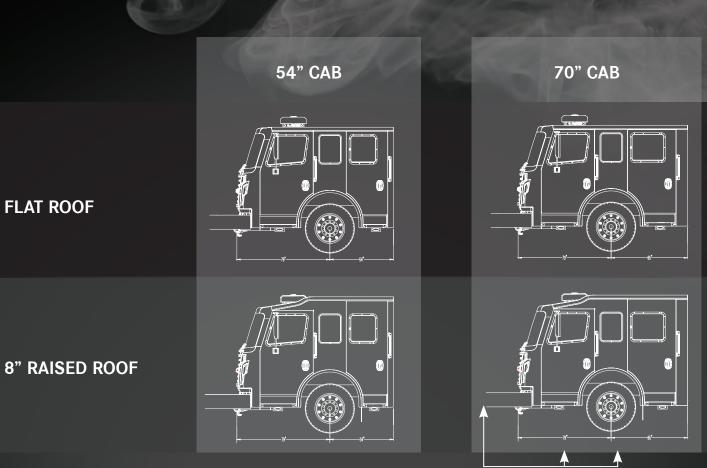
79" Dimension is from "Face of Grille to Centerline of Front Axle.
