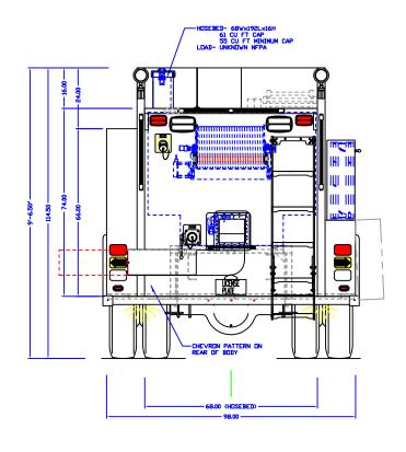
1. OVERALL HEIGHT IS IN LOADED CONDITION. UNLOADED HEIGHTS MAY BE 4" ABOVE HEIGHTS SHOWN.
