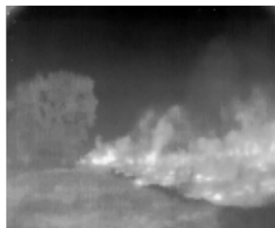
Visual and thermal image comparison shows hot-spot detection along the fire edge
