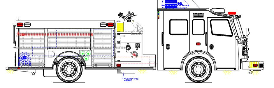
CHASSIS: COMMANDER 6511 HALE 1500 GPM PUMP: POLY/750/20(FOAM) PANEL MATL:LINE X TOP-S/S SIDES COMP INTERIOR: LINE X
