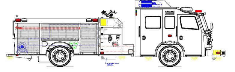
CHASSIS: COMMANDER 6511 HALE 1500 GPM POLY/750/20(FOAM) PANEL MATL:LINE X TOP-S/S SIDES COMP INTERIOR: LINE X PROPRIETARY AND CONFIDENTIAL
