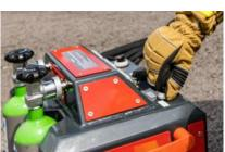
6) The flushing time depends on the size and architecture of the battery and can be between 10 and 60 minutes.
